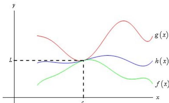
FIGURE 3.0.2. The sandwich Theorem
