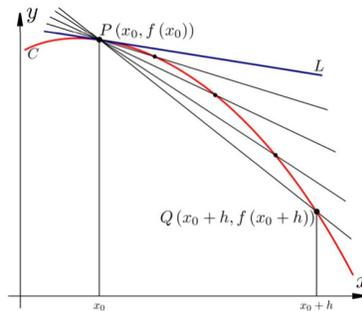
FIGURE 4.0.5. Secant line approaching tangent line
